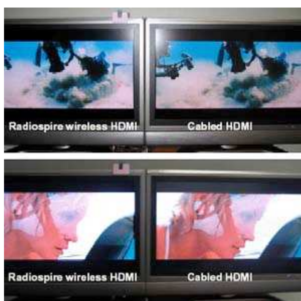
Figure 3: Comparison of the video quality between the wired and wireless links revealed no visible differences under any of the test conditions, for any antenna orientation and with obstructions in the beam.
